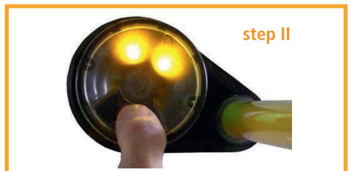
Fig. 6 Switching the phase comparator on / step II
