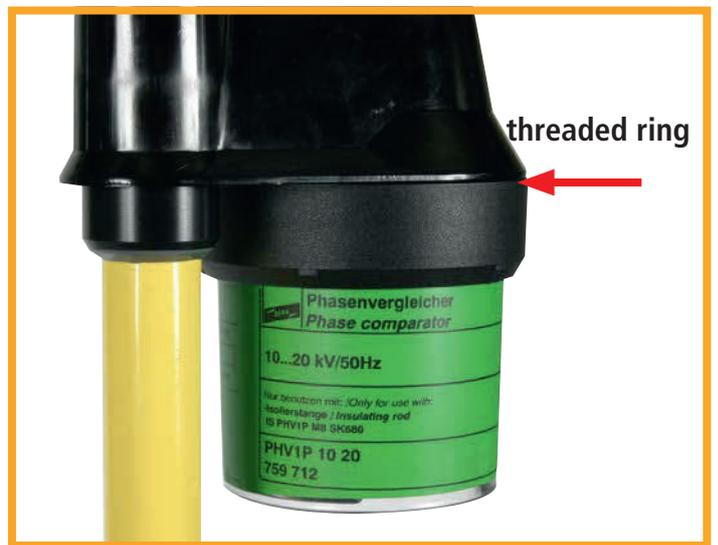
**Note:** Tampering with (except battery replacement) and modification of the phase comparator are not permitted. Non-operational or damaged phase comparators must be removed from service.
